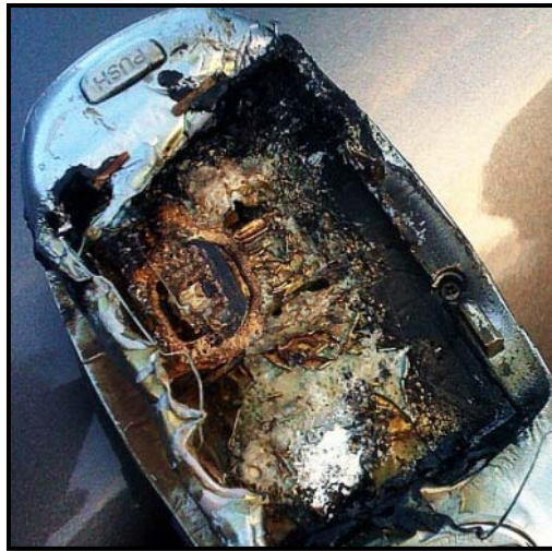
Exploding counterfeit cell phone battery
